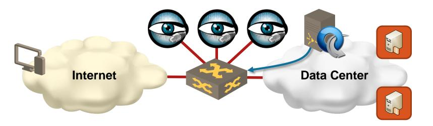
OpenFlow used to distribute the load to multiple IDS appliances
