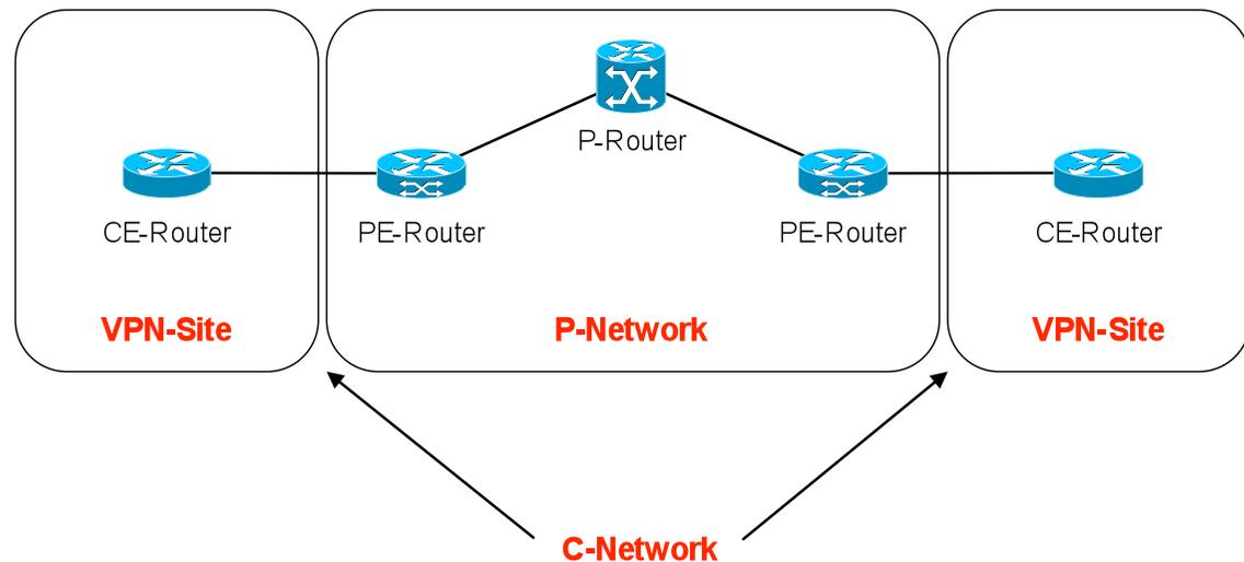
During transport two labels are used: one to identify the 'egress PE', the other one to identify the customer/a particular VPN.
